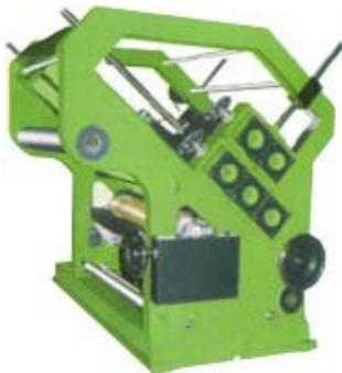
Modern single facers must be flexible enough to change flutes quickly to allow the plant to meet the customer's needs without excessive downtime.
