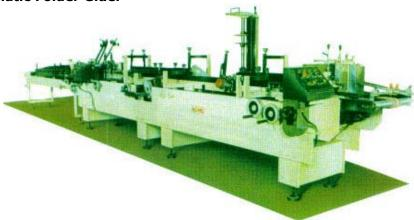
It is a folding cum Gluing machine for the manufacture of cartons in packaging of Pharmaceuticals products, Food Stuff, Detergents and many other products.
